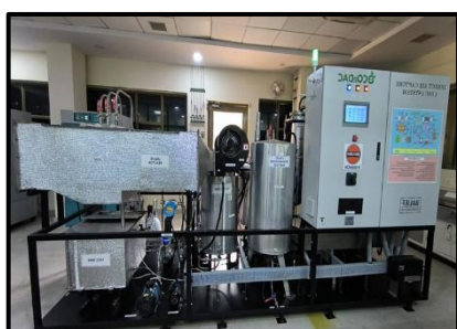
Fig.3. Integrated Direct Air Capture (DAC) Pilot plant for CO 2 capture and its utilization in microalgae growth.
