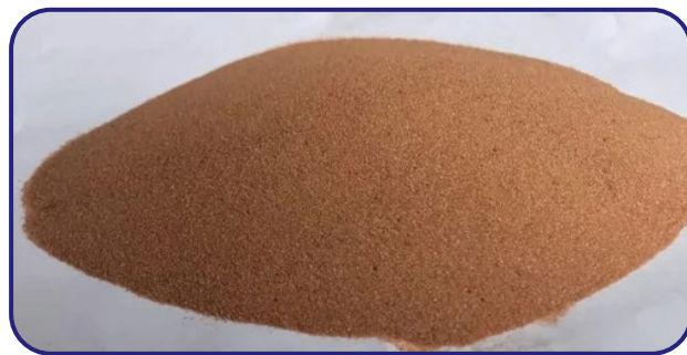
Reclaimed Core sand (Reclaimed using Thermal Reclamation process)
