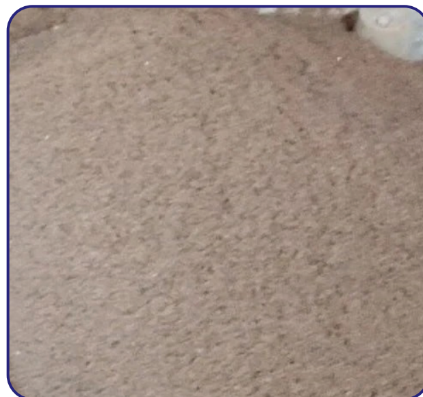
Reclaimed CO2sand (Reclaimed using Mechanical Reclamation process)
