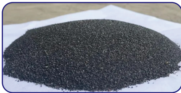
Reclaimed green sand (Reclaimed using Mechanical Reclamation process)
